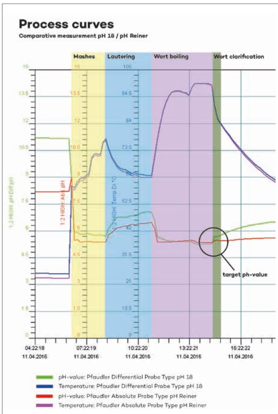
Fig. 2: Comparative measurement diagram in the mashing and wort process at Weldebräu using Pfaudler absolute and differential pH probes
