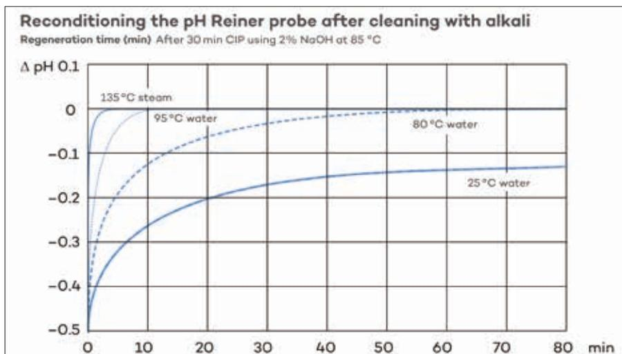
Fig. 1: Reconditioning the pH Reiner probe after cleaning with alkali
